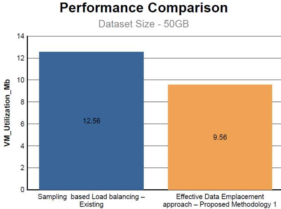
Figure 8: Performance Evaluation of the EDEC approach against SLB approach in terms of VM Utilization
